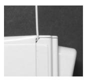
3) Leave the antenna pointed straight up, or bend antenna back and down to conceal antenna once mounted. Continue with mounting and RF testing in final mounting location.
